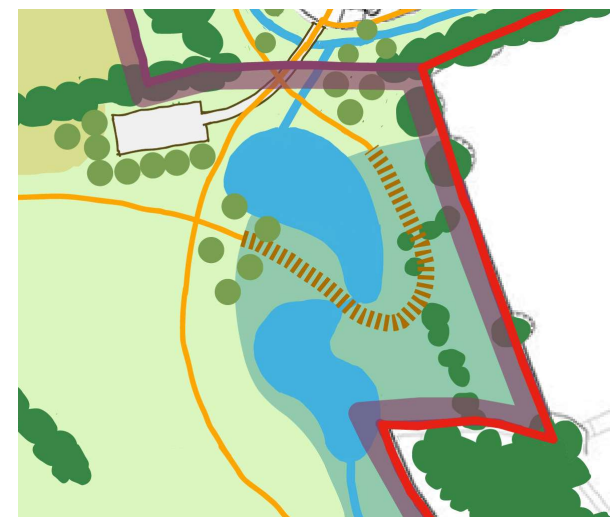
Figure 3.6: Swales carry water to attenuation ponds which both mitigate flooding, provide amenity and enhance biodiversity
